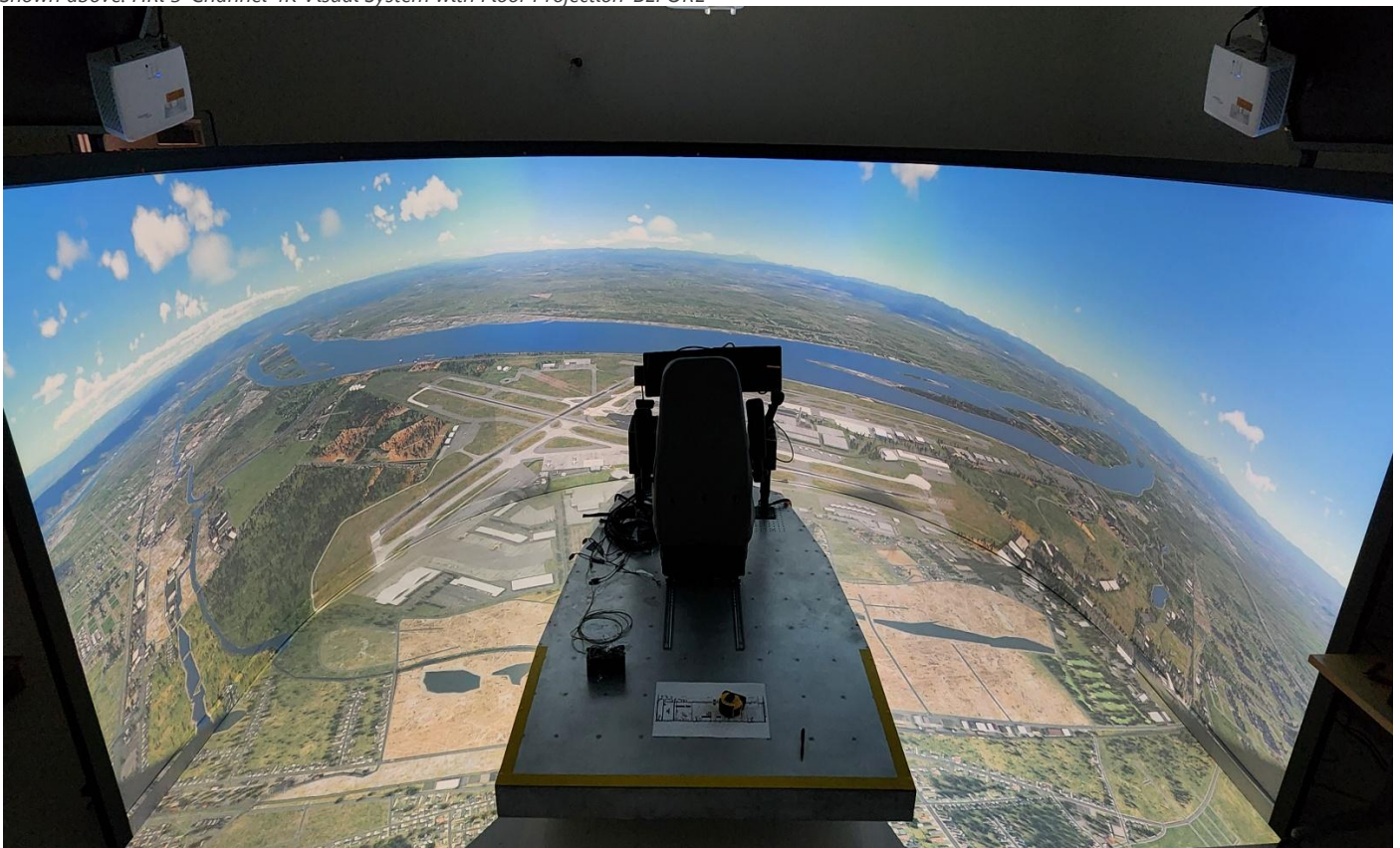
Shown Above: HRI 5-Channel 4K Visual System with Floor Projection-AFTER
